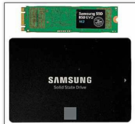
↑ The size difference between M.2 (top) and SATA (bottom) SSDs can clearly be seen.
